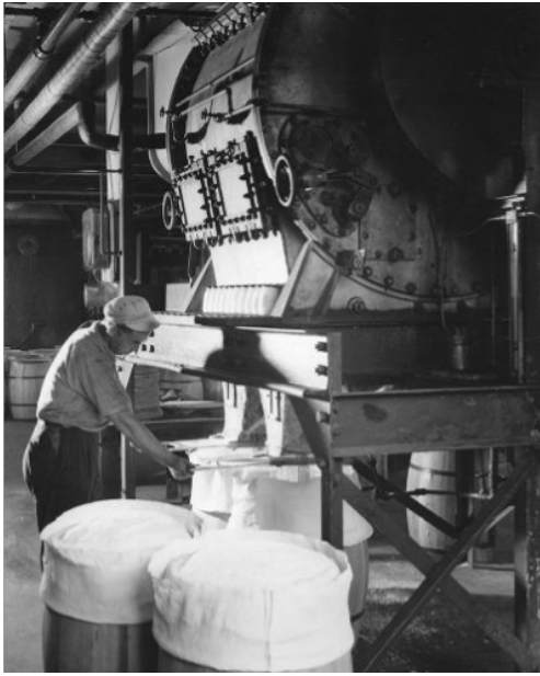
Camphor flaker machine, Dupont's New Jersey factory. 1941.
